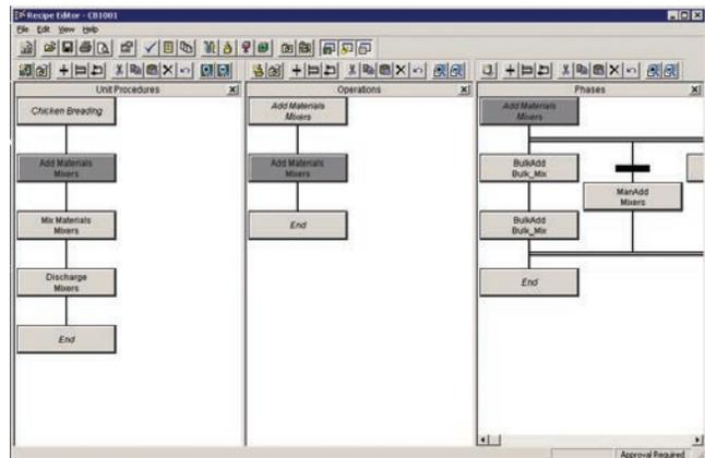
The InBatch Recipe Editor uses the information in the process model and materials management as part of recipe procedure development. An InBatch master recipe may or may not be size specific, and can be assigned to any process line that has fits the equipment requirements defined in the recipe. All formula quantities for ingredients, intermediates, by-products, and finished goods are configured as either actual quantities or scalable as a percent of the batch size.
