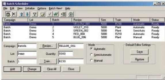
A batch is scheduled by entering campaign, lot, and batch ID, as well as the desired batch size. A Recipe as well as the train need to be selected. When the batch size entered is greater than the defined maximum batch size of the recipe, the Batch Scheduler opens a dialog box to confirm the splitting into multiple batches. Once confirmed, the proposed number of batches is automatically generated and are added to the list.
